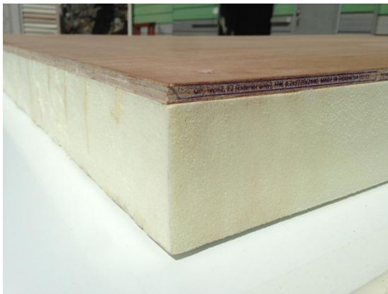
Floor Panel (Plywood-XPS-Al)
